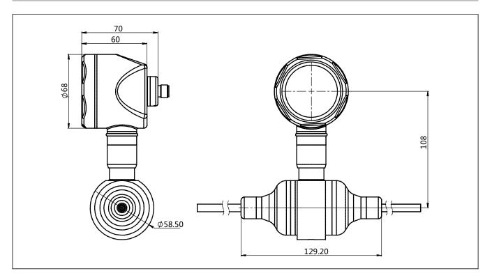
Drawing and dimension with display (C) / without display (A) horizontal installation (F2) (unit: mm)
